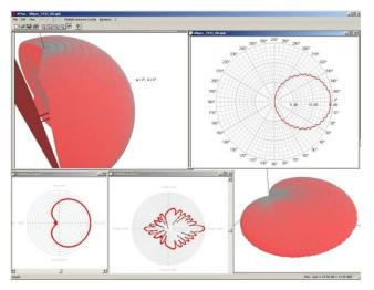
(MASC). This feature takes into account the superposition of multiple antennas radiating the same signal (including phase shifters and power splitters) as well as the consideration of the local environment (masts, arms, walls, sub-arms, etc.) to determine the actual antenna pattern.
