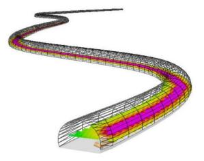
CellTunnel allows the definition of different cross sections within one tunnel. Additionally multiple curves with different radii can be defined to model the tunnel and its curved profile accurately. Additionally, the terrain profile inside the tunnel can also be defined in CellTunnel.
