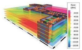
path loss and wide-band properties, such as delay and angular spread, LOS/NLOS, directional channel, impulse response, angular profile, and propagation paths, of radio links within buildings.
