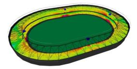
The pixel databases are generated with individual, scanned bitmaps of the drawings of each floor. Different material properties and heights of the objects can be assigned to the various colors in the bitmaps.
