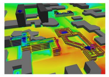
order to determine the parameter sets of the base transceiver stations (or access points). With the introduction of MIMO and wireless broadband services, the wideband properties (e.g. delay spread, angular spread and impulse response) of the mobile radio channel become more and more important for the network planning.
